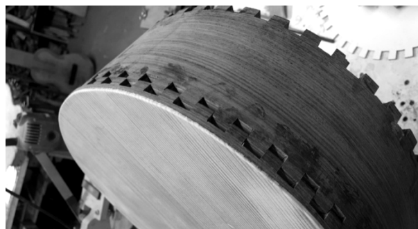
Fig. 1 The notched connection of ribs and plates
